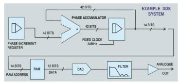
A DDS generator can be swept over a much wider frequency range than an analogue generator and can perform phase continuous frequency hopping.
