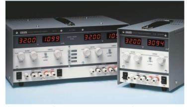
Specifications for Main Outputs: Line & load regulation <0.01%. Output noise <1mV rms. Meter accuracies  $0.1\% \pm 1$ digit - voltage,  $0.3\% \pm 1$ digit - current.
