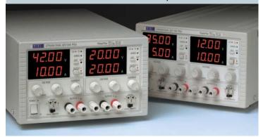
Line regulation <0.01%. Load regulation <0.02%. Output noise <2 mV rms. Meter accuracies:  $0.2\% \pm 1$  digit - voltage,  $0.5\% \pm 1$  digit - current.
